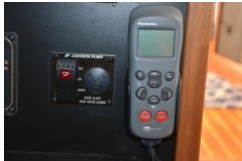
Bilge/High Water Alarm & Autopilot Remote
