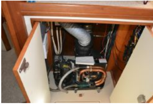
Aft A/C compressor
