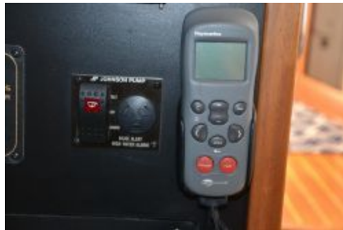
Bilge/High Water Alarm & Autopilot Remote
