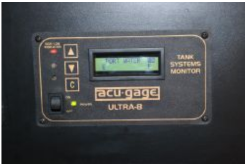
Water Tank Monitor
