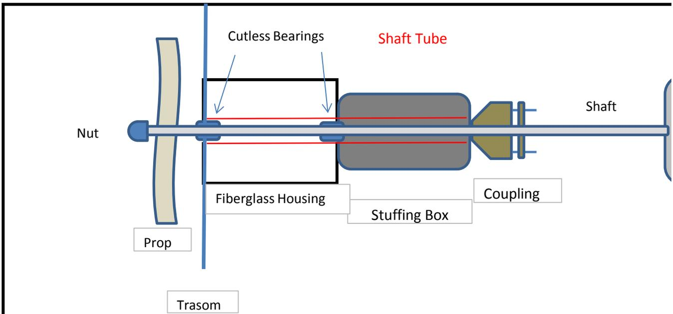
Water flowing through cutless bearings but not reaching coupling even with 50% of packing removed
