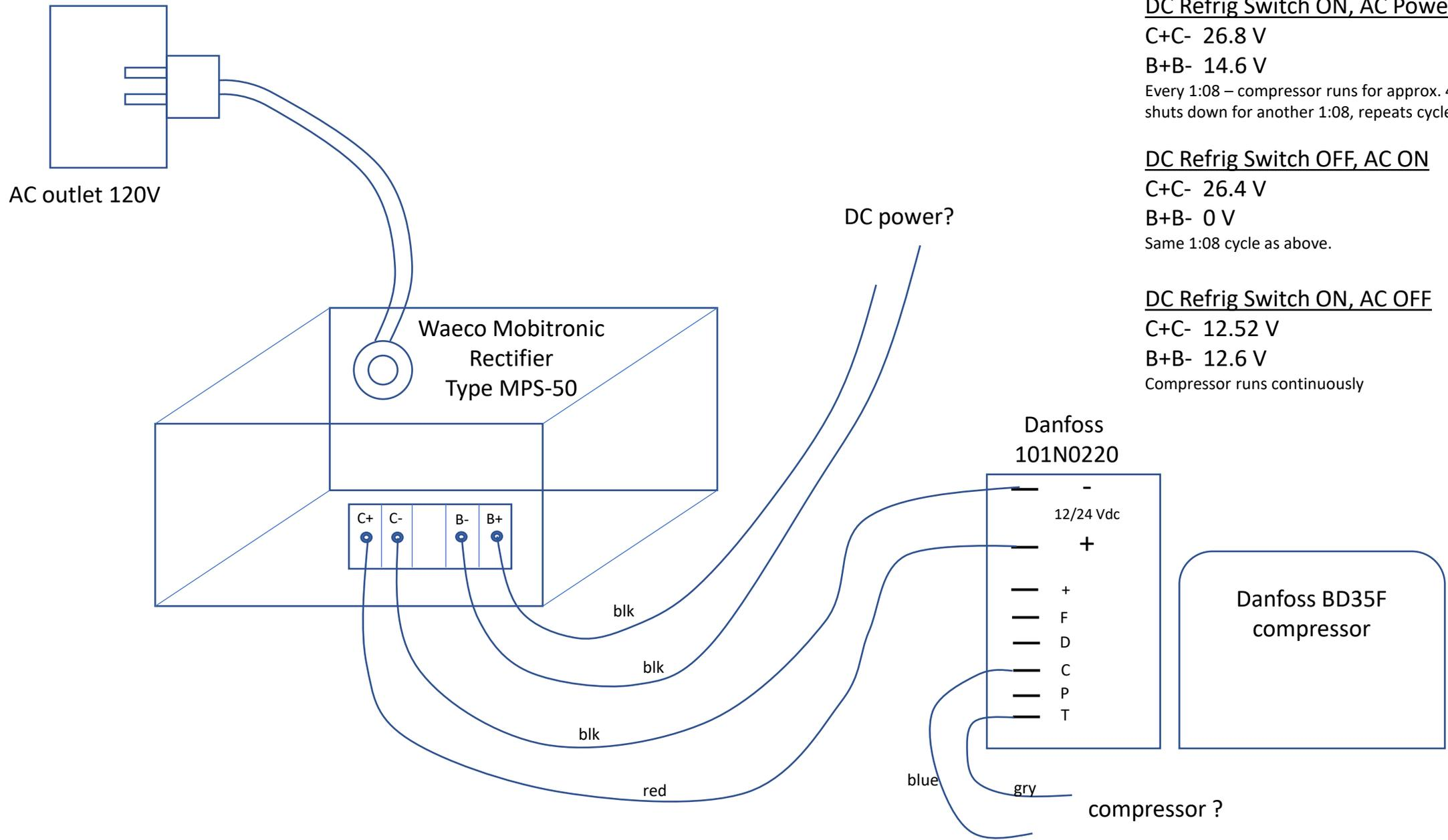
DC Refrig Switch ON, AC Power ON
