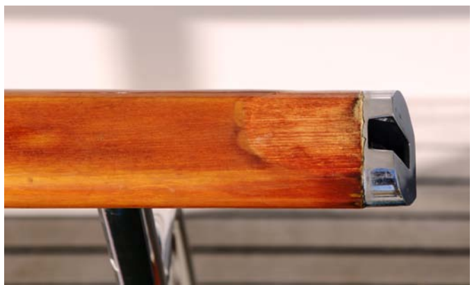
The stainless gate hardware covers the end grain of the wood, a critical area where the fibers soak in moisture. The hardware should be removed, the end grain sealed with epoxy, and new bedding compound applied.
