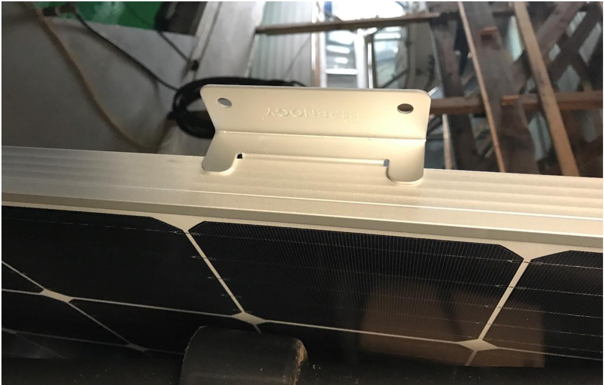
3. **Where should they be mounted?** Here's where it gets a bit tricky. Shading is the #1 cause of panel inefficiency. As little as one corner shaded by a mast, boom, radar or flag will cause degradation of output. As vessels are in a constant state of motion it is nearly impossible to eliminate this problem so any location will be a compromise. Pick the highest and least affected areas to mount your array.
