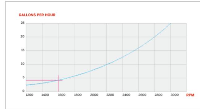
At 1450 RPM the higher horsepower engine will burn 2.7 GPH. Given the running speed of 7 knots at 160 HP, we arrive at a fuel burn of 2.6 nMPG—a 30% improvement over the smaller engine.
