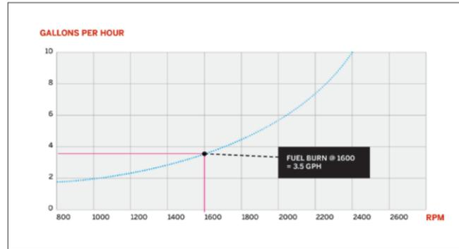
At 7 knots we will burn 3.5 GPH, resulting in a fuel economy of 2 nMPG. We can compare this performance to a larger engine, increasing from 210 hp to 370 hp. In the following engine performance specs (*graph, top-right*) we see that this engine will need 1,450 RPM to produce the same 160 hp.
