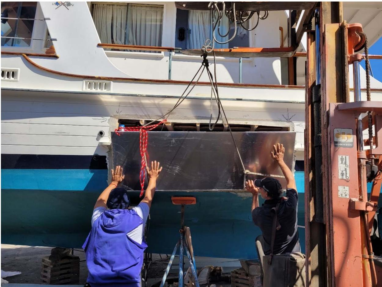
The tanks were then epoxy coated, installed and secured:
