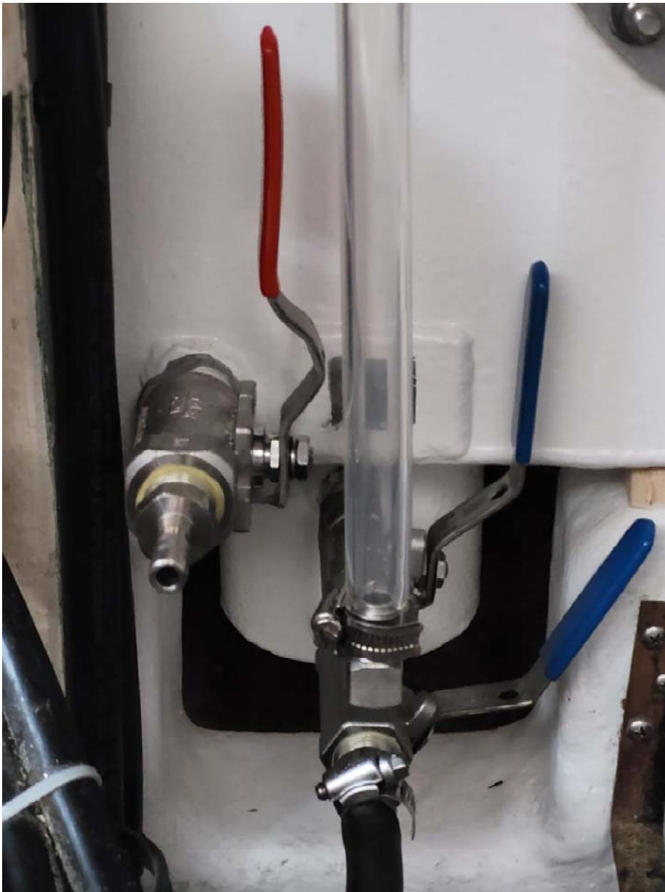
I replaced (90%) of the original hard copper fuel tubing with A1 rated hose.
