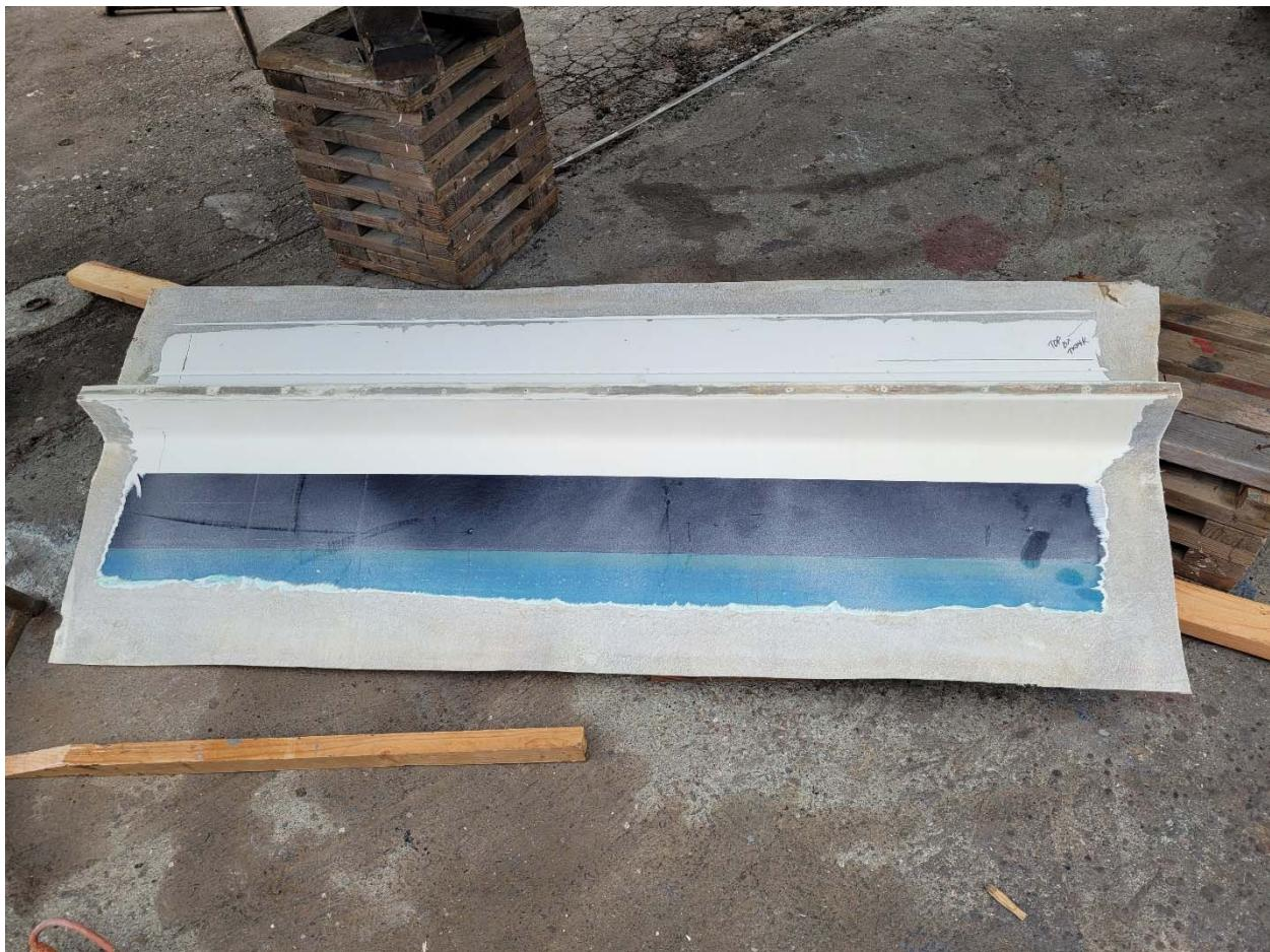
A blend of brute force grunt work and finesse is involved in removing the plugs (stb side pic) due to internal bracing etc. Note: secondary FRP bonds are way easier to break than one might expect.
