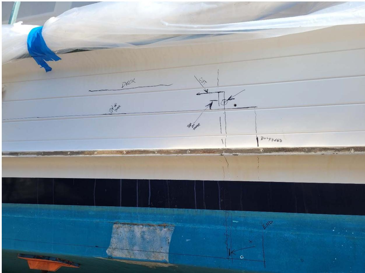
Next you prepare to remove the patch area to get to the tanks. This starts with grinding a wide (compared to the cut line) shallow Vee, centered on where the cut will eventually be, into the hull. The wide Vee becomes the area that provides the scarf ratio for later re-lamination.
