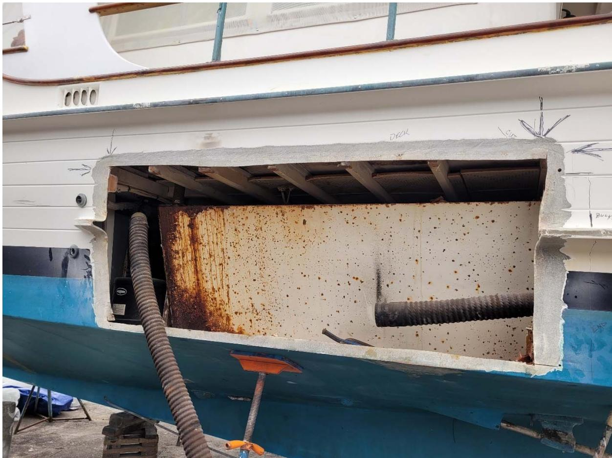
Combine 38 years, a suspected past leak at the deck fill fitting, steel tanks, and this is the result:
