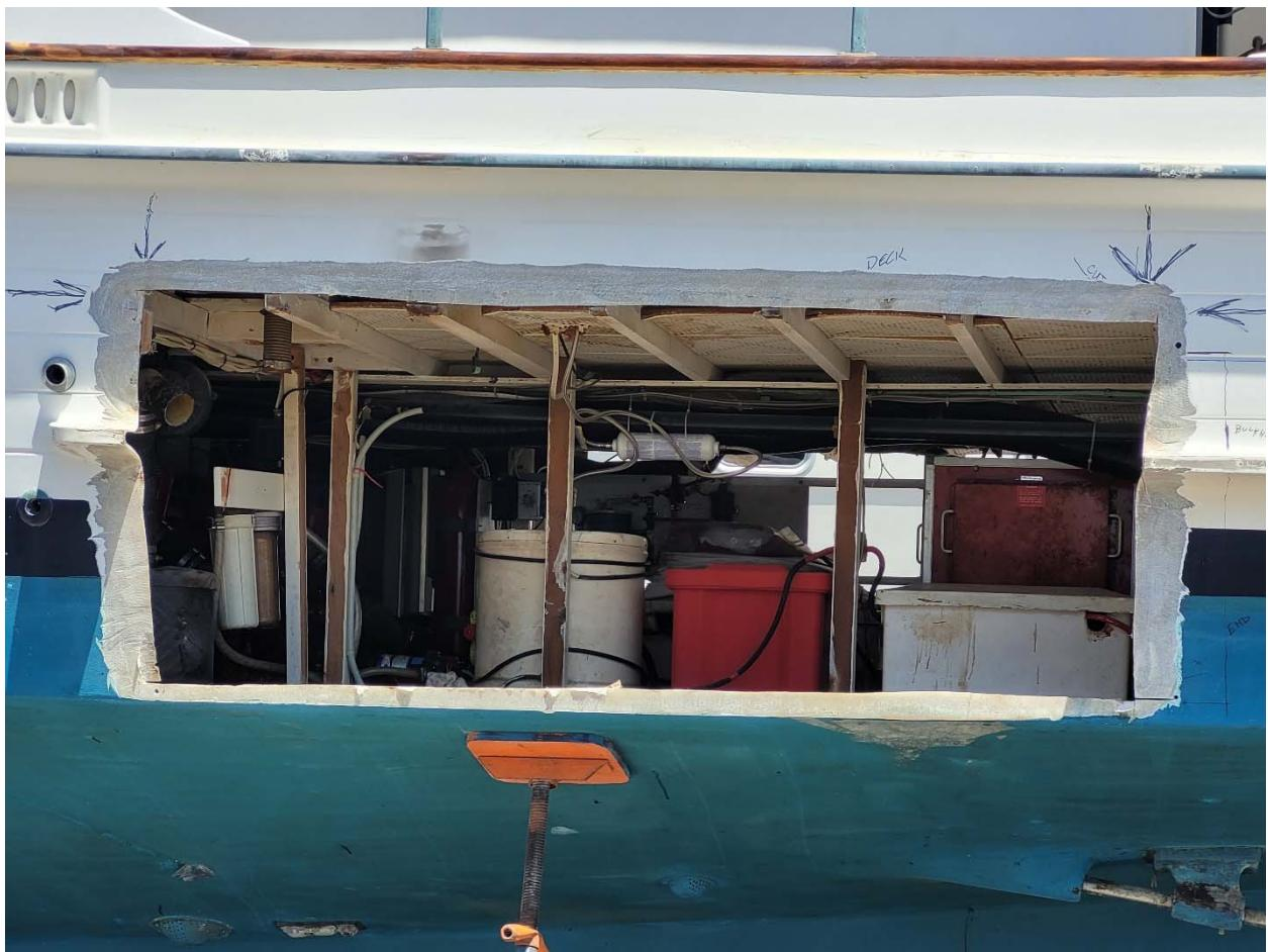
Moral of the story? That little bit of caulking around deck fills is really important! It's much easier to redo it periodically than to replace tanks! You can bet we re-bedded all the deck (fuel and water) fills.
