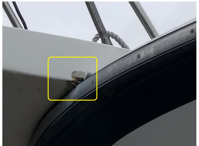
Cracked pulpit, port and starboard
