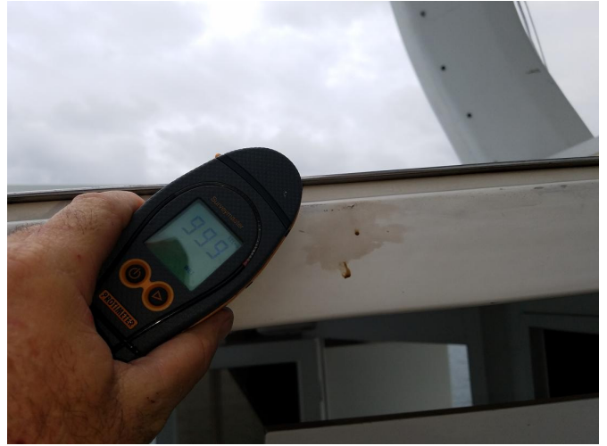
Moisture meter pegged 999 (0-999) scale, slider for bridge / aft deck access
