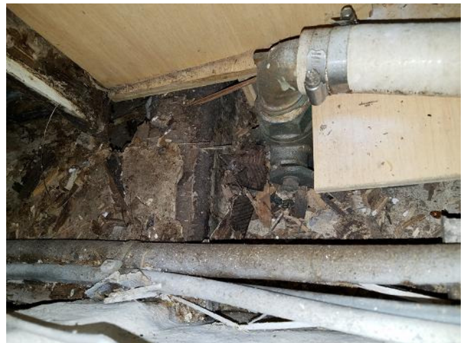
Deteriorated shelf, inside aft marine head vanity
