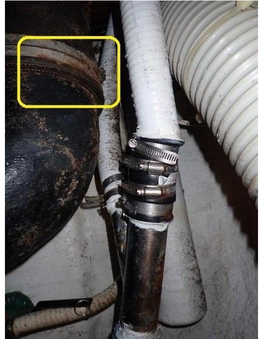
Drain assembly homemade/leaking, aft engine compartment note corroded exhaust hose clamps
