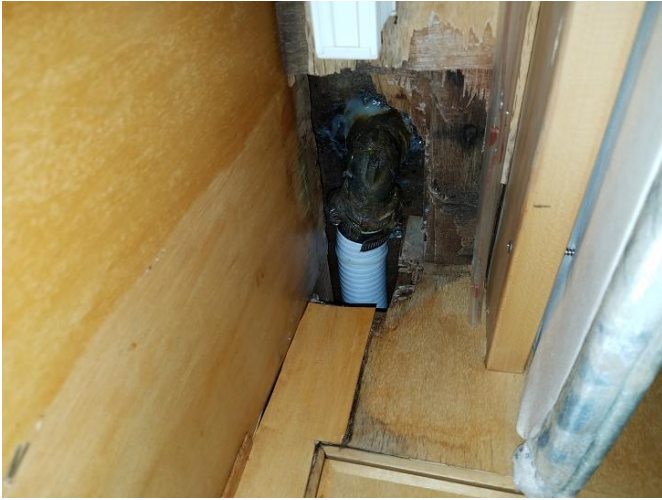
Looking up, starboard aft salon corner water damages from above
