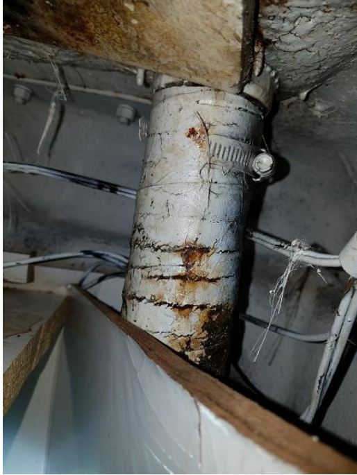
Age/jacket cracks for aft deck drain hose, port aft corner
