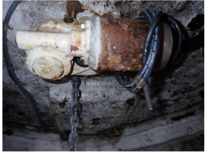
Windlass motor, heavy corrosion
