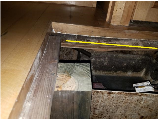
Master stateroom sole soft, supported by wedged 4 x 4
