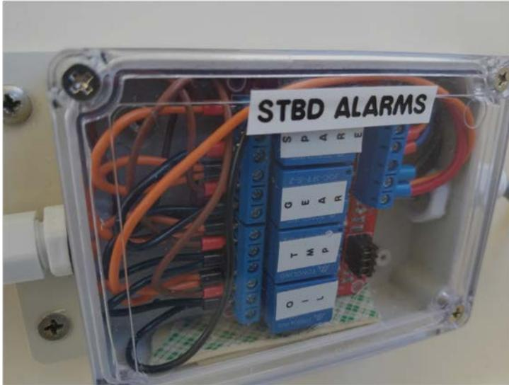
The next issue I had to work thru was how to power everything. I originally powered the Maretrons, 7607, Chetco and relay boards from the helm supply using a small fuse panel for supply and ground. Everything worked great, except the alarms were on whenever the helm supply was powered. Not good. So, the Chetco and relays are powered from each engine's on switch. The 7607 is on the helm supply and the Maretrons are powered from the NMEA network which is on the helm supply also.
