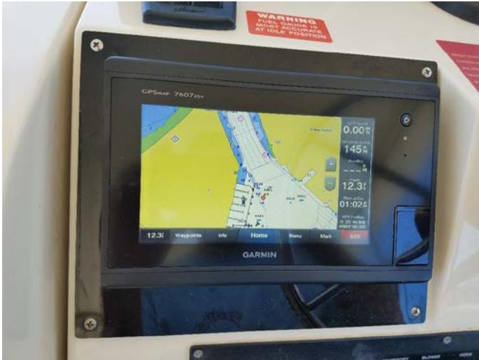
Here is the overall new layout. The black acrylic panels mounting the new gear, and covering old holes were ordered custom from BoatOutfitters.com
