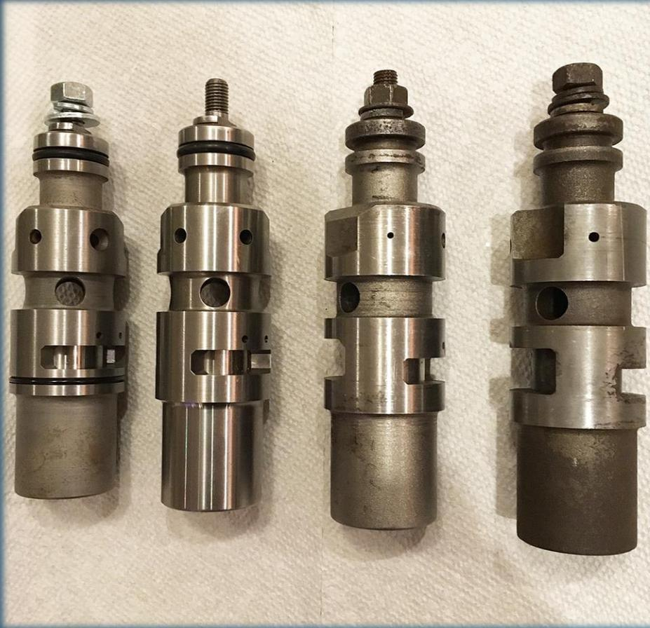
Interesting to note the improvements made to the control valve over the years. More and larger ports for better lubrication and more flow to the clutch pistons.
