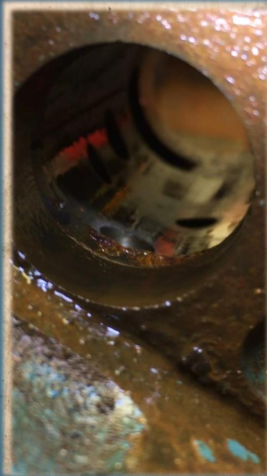
Inside view of a control valve bore showing buildup of rust and sludge.
