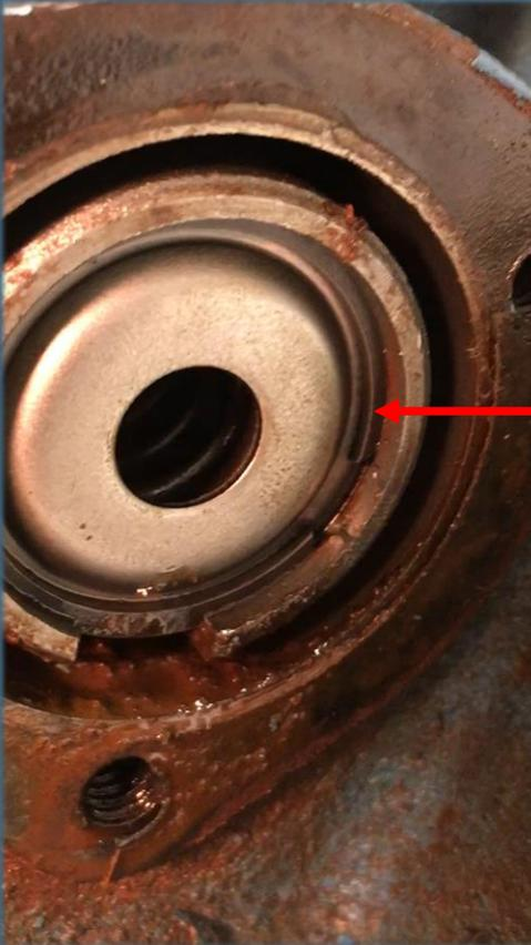
Removal of the cover plate and cam reveals the end of the control valve. Note the rust and buildup of sludge.
