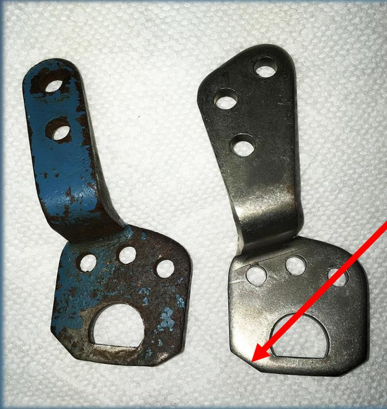
A subtle change in an angle means the shift lever can't go past the forward position ensuring full flow of ATF to the forward piston.
