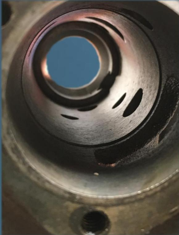
Clean out the bore with Scotch Brite, scrape off the old gasket, and you're ready for reassembly.
