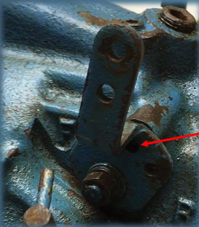
After removing the linkage from the top of the shift lever, remove the 7/16" nut.
