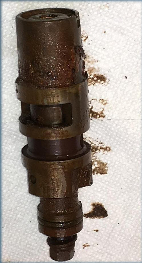
This control valve still shifted the transmission, although the front seal was blown. This is a good example of what happens when you do not change zincs in the heat exchanger. When the oil cooler corrodes, the transmission fills with water and starts rusting out.
