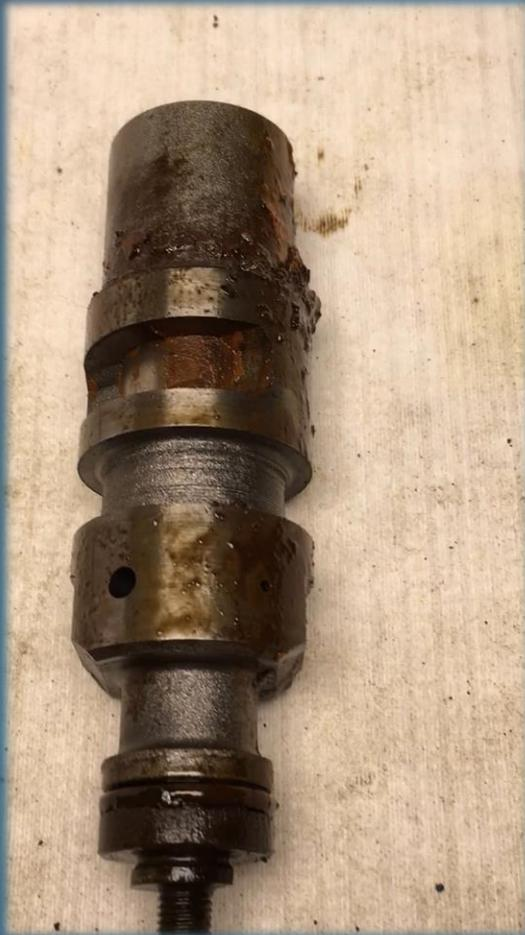
View of a removed control valve. The regulator valve was frozen so this transmission would not have been able to relieve excess pressure into the sump.
