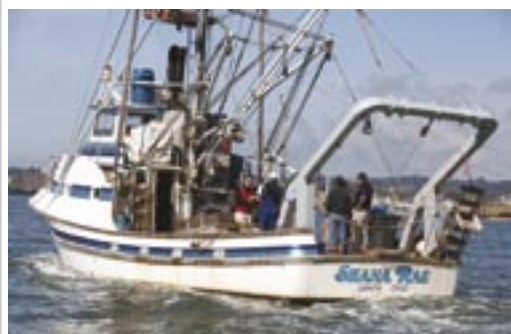
Our powerful test boat was Shana Rae , a 48ft research vessel with a 375hp Caterpillar engine driving a 40in prop, which simulated gale-force pulling power
