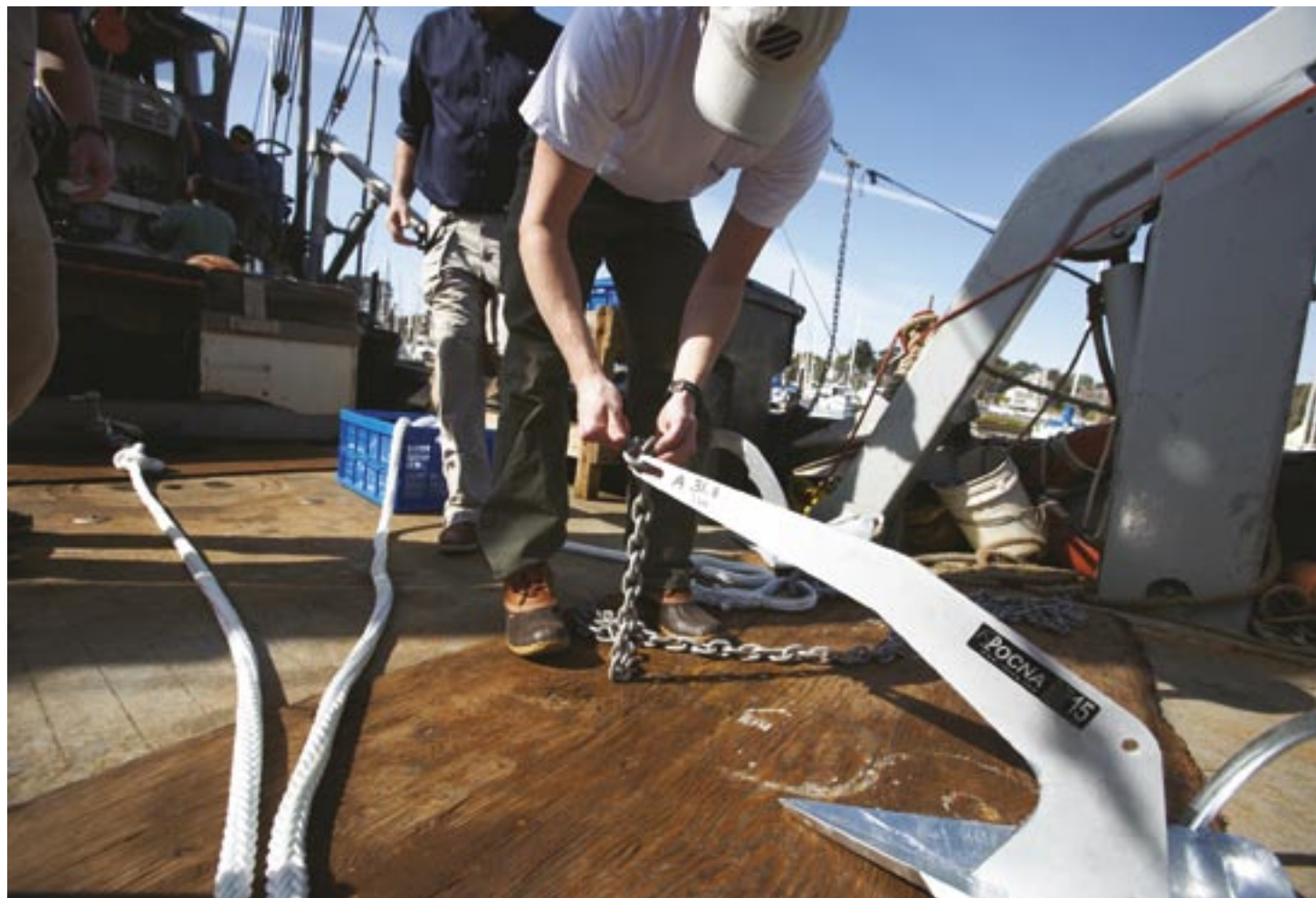
Each anchor was attached to 20ft of 5/16 inch chain cable and 108ft of 12-strand 1in nylon rope for the 5:1 scope test, and then lowered into a depth of 20ft
