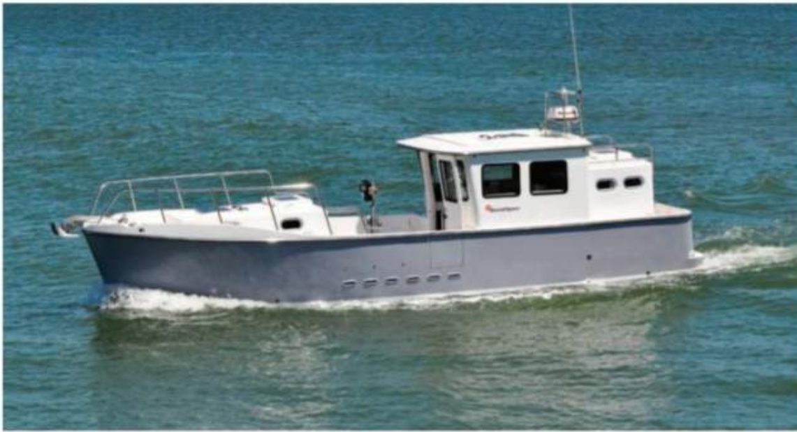
While it can reach 9.8 knots easily, the SeaPiper 35 excels at around 6.5 knots, where its range stretches beyond 2,000 miles.
