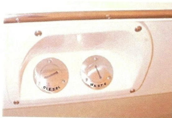
Stbd. Side Fuel Fill & Waste Clean Out
