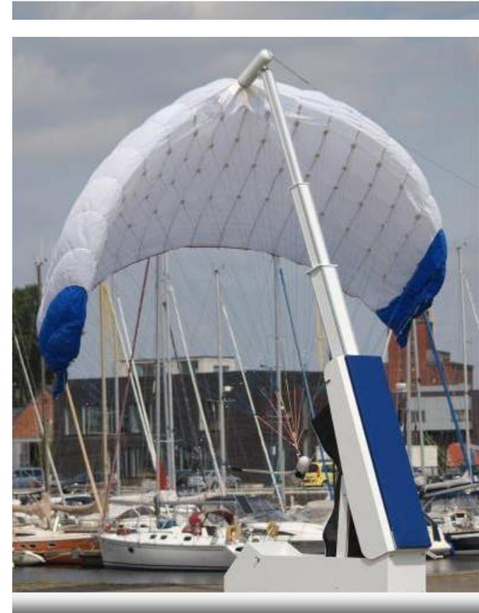
The launch and recovery system of the SkySails propulsion manages the deployment and lowering of the towing kite and is installed on the forecastle. During launch a telescopic mast lifts the towing kite, which is reefed like an accordion, from its storage compartment.
